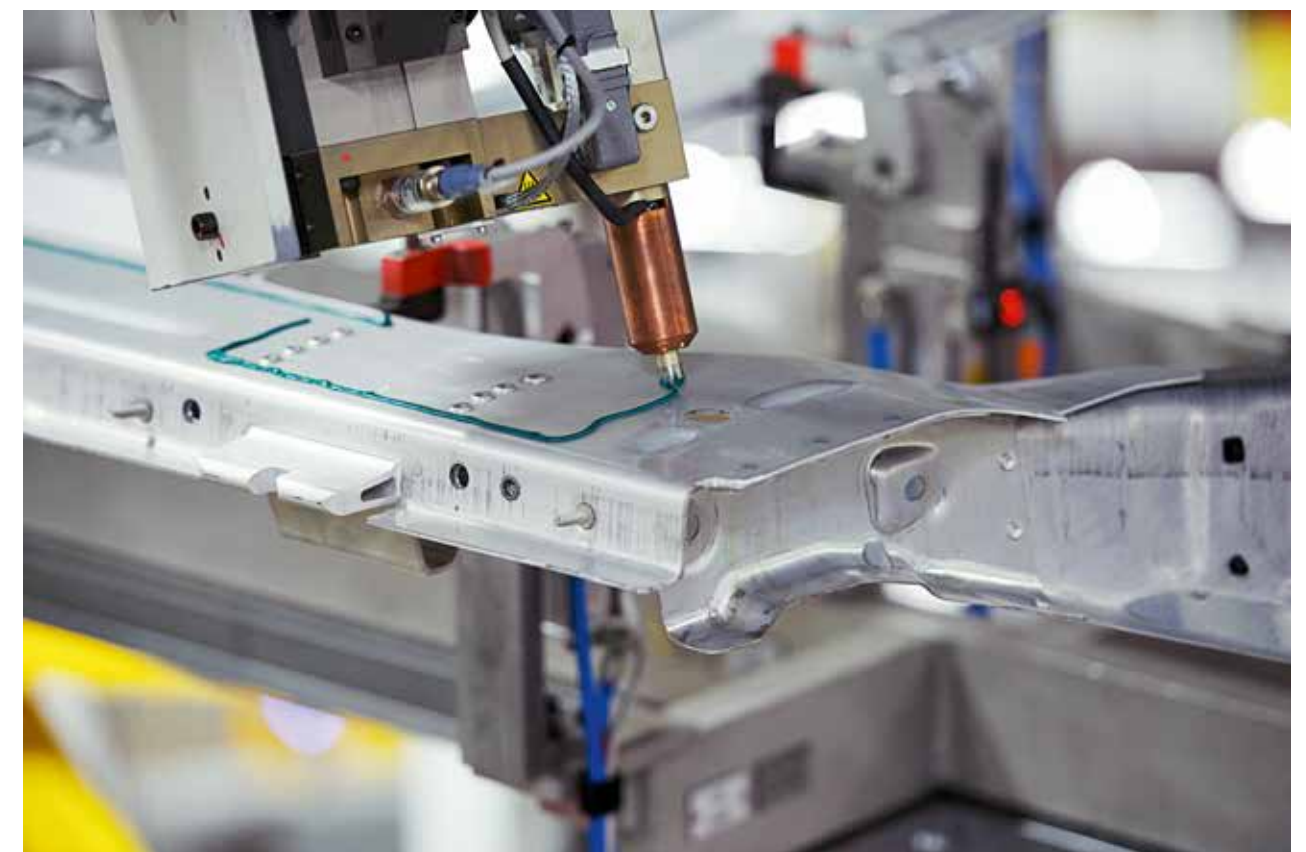
The trend toward lightweight structures in car body construction also opens up a new broad application in the field of elastic adhesives.
